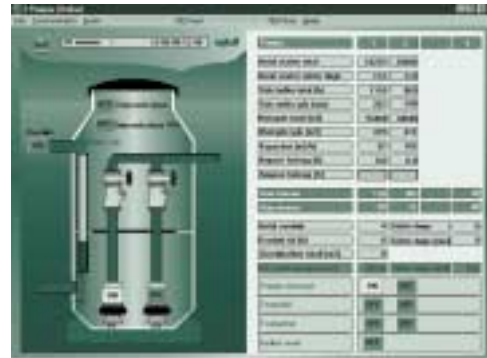
From MJK-Link™: Pump station with 2 pumps and overflow.
