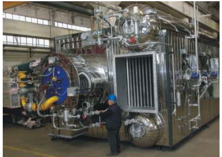
CT 20 t/h in package configuration
