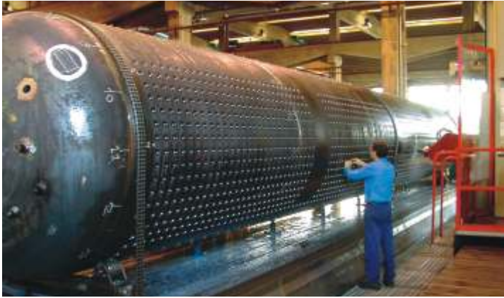
CT steam drum under machining
